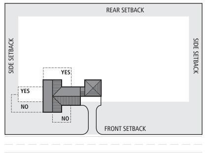
Figure 1-01. Additions to Nonconforming Structures
